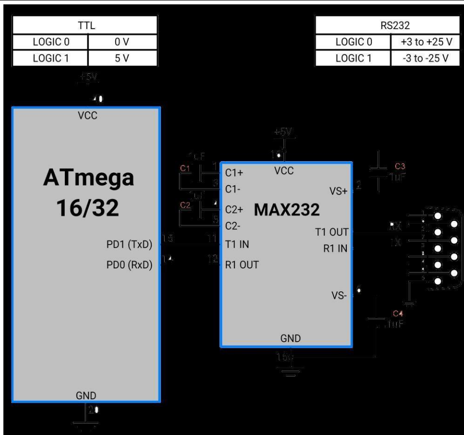
ATmega16/32 Serial Interface Connection Diagram
